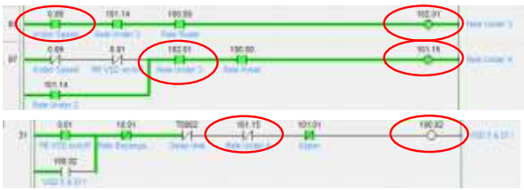
Gambar 37. Diagram ladder kondisi under speed
