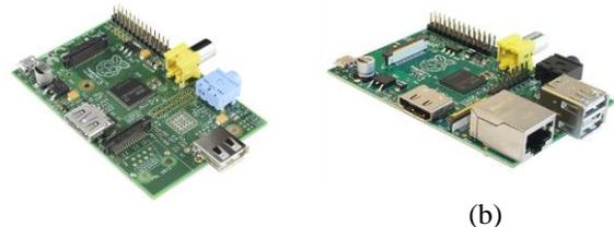
Gambar 1. (a) Raspberry Pi Model A (b) Raspberry Pi Model B
