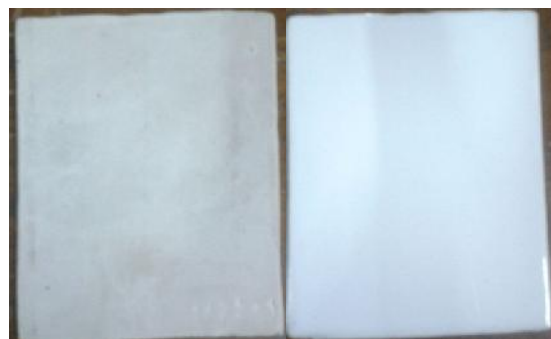
Gambar 2. Sampel Bahan Isolator Keramik 20 KV
