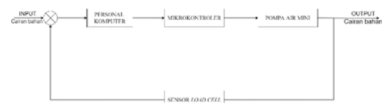
Gambar 3 diagram blok sistem proses pengisian tangki buffer
