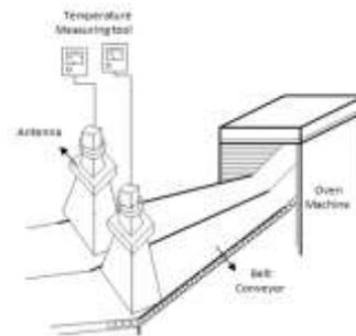
Figure 7.1 Antenna in radiometer measurement system.
