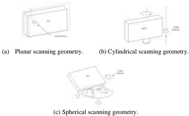
**Figure 5.6 Near-field scanning geometries for close-up measurements of an aperture antenna.**
