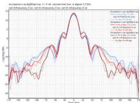
Figure 7.3 Cartesian plot of directivity for configuration 1.
