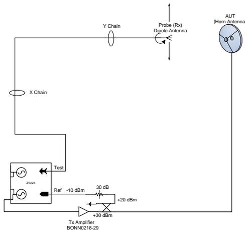
Figure 6.4 Schematic of near-field measurement system.
