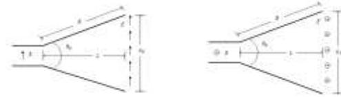
(a) E-plane cross section (b) H-plane cross section
