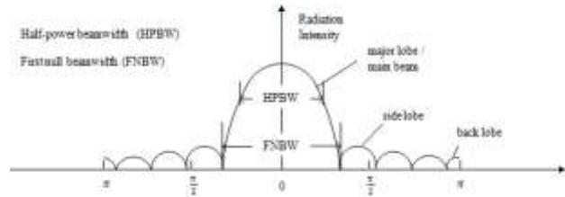
**Figure 4.2 Linear plots of power pattern and its associated lobes and beams [1].**
