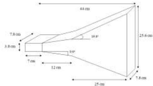
**Figure 6.3 Horn dimension in configuration 1**
