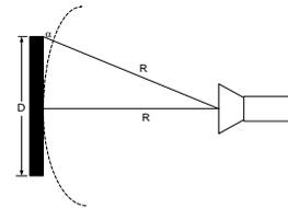
**Figure 5.5 Phase error at antenna edge.**
