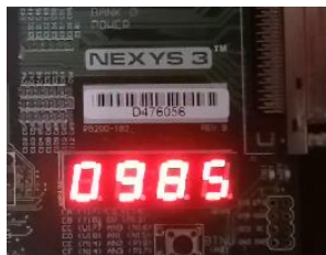
Gambar 8. Tampilan Counter Seven Segment jika Limit Switch Lajur Utara = 0.
