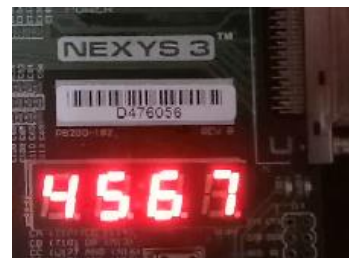
Gambar 10. Tampilan Counter Seven Segment jika Limit Switch Lajur Utara = 1.
