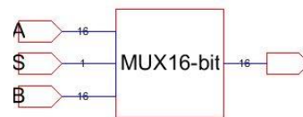
Gambar 5. Skematik Multiplexer 2-ke-1 16-bit
