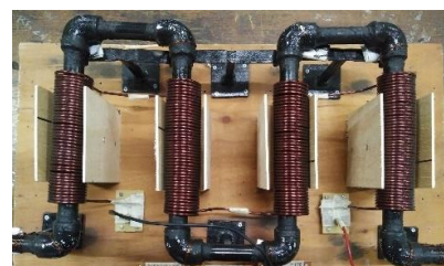
Gambar 8 Realisasi beban kerja ( load ) pipa stainless steel
