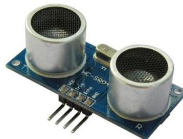
Gambar 5. Sensor Ultrasonik
