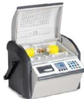
Gambar 3 Alat uji tegangan tembus (*DPA 75C Oil Breakdown Measurement*)
