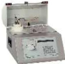
Gambar 4 Alat uji permittivitas relatif ( *DTL measuring system* )
