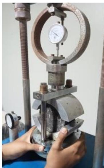
**Gambar 3.** Pengujian *marshall test*
