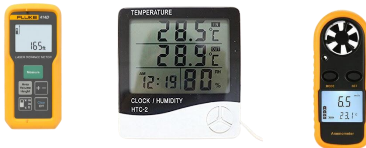
Gambar 3. Alat ukur (a) Laser distance meter ; (b) Digital clock thermo-hygrometer ; dan (c) digital anemometer
