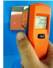
Gambar 6. Pengukuran Steel Temperature
