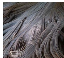
Gambar 2. Besi cor ( Reinforce Mesh ) ukuran diameter 6 mm
