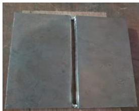
Gambar 3. Sambungan Single V Butt Joint 60°
