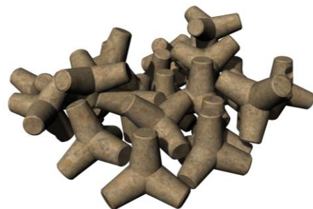
Gambar 5. Tampak Perspektif Model Submerged Breakwater
