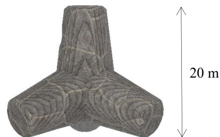
Gambar 6. Dimensi geometri breakwater .
