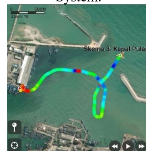
Figure 17. Recorded Travel Route History during Scheme 2 Testing on Fishing Vessel by the Comparison GPS.
