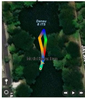
Figure 2. The recorded travel route history during testing in Scheme 1 Model Vessel by the comparison GPS.
