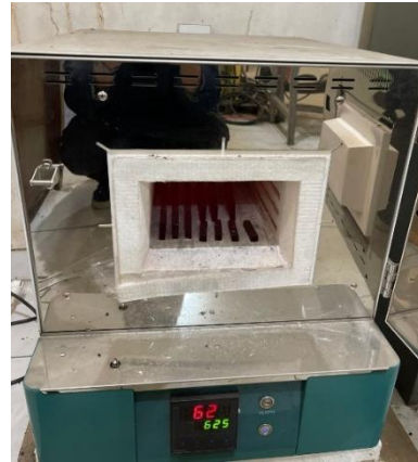
Gambar 5. Proses PWHT Annealing
