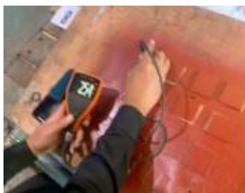
Gambar 11. Proses Perhitungan DFT
