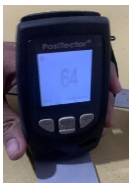
Gambar 7. Pengecekan surface roughness
