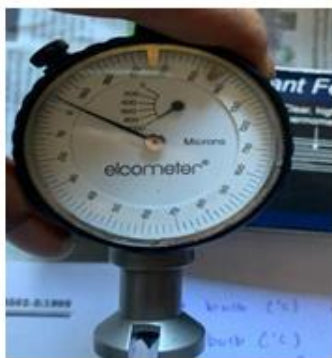
Gambar 3. Alat Roughness Meter
