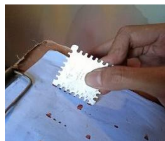
Gambar 10. Proses Perhitungan WFT
