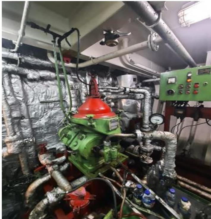
Gambar 2 Gambar *Fuel Oil Purifier* Kapal MT. Cordelia W
