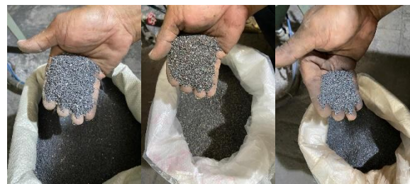
Gambar 3. Material Abrasif ( Steel Grit , Garnet , Aluminium Oxide )
