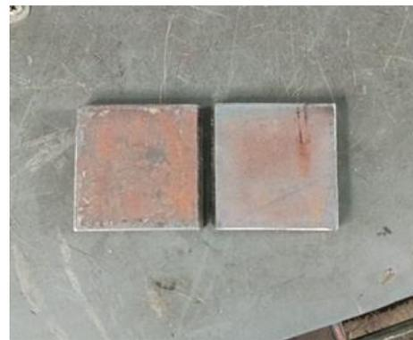
Gambar 1. Baja ASTM A36
