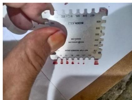
Gambar 13. Proses Perhitungan WFT
