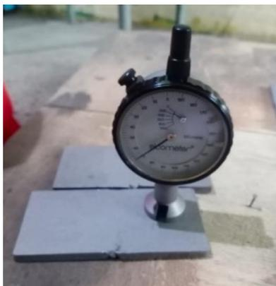
Gambar 9. Alat *surface profile gauge*
