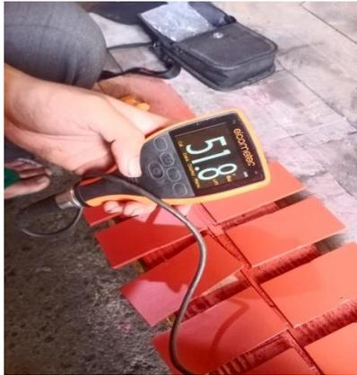
Gambar 14. Alat Dry Film Thickness Gauge
