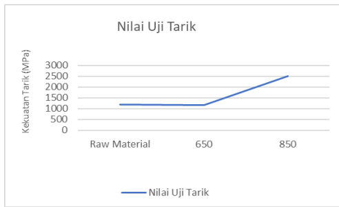
Gambar 8. Diagram rata-rata tegangan tarik
