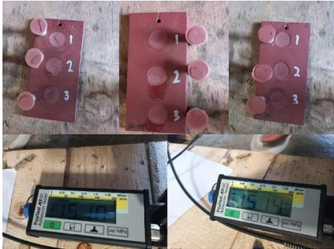
Gambar 5. Hasil Pull Off Test & Dolly
