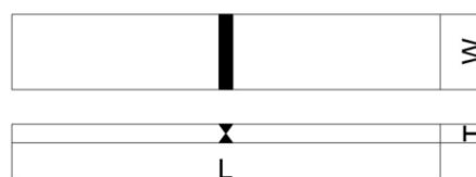
Gambar 5. Spesimen uji tekuk (ASTM E19014)
