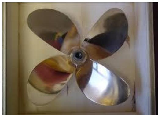
Gambar 1. *Propeller* B4-70
