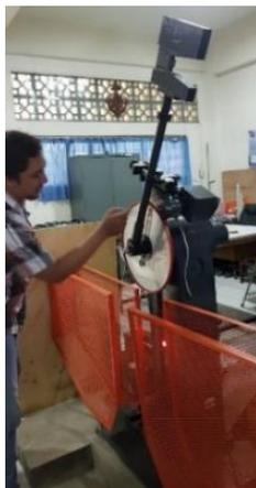
Gambar 5. Alat Uji Impak
