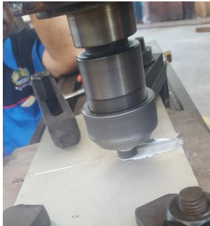
Gambar 2.. Prinsip Friction Stir Welding
