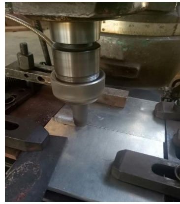
Gambar 1. Prinsip Friction Stir Welding
