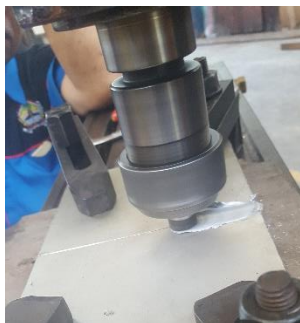
Gambar 1. Prinsip Friction Stir Welding
