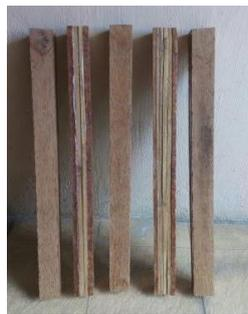
Gambar 5. Balok Laminas
