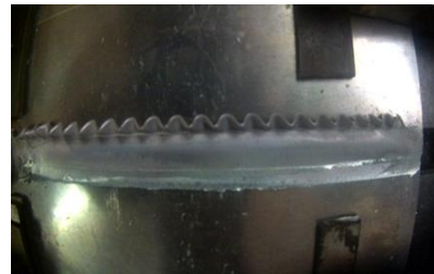
Gambar 9 Hasil pengelasan friction stir welding
