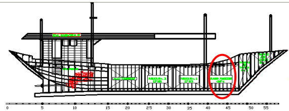
Gambar 3. Lines Plan Kapal Perikanan 30 GT
