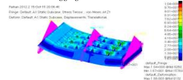
Gambar 6. Output Result Stress Msc Patran Kondisi Sagging 2
