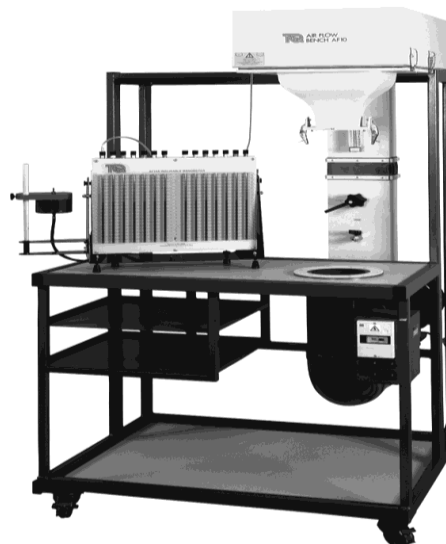
Gambar 2. Air flow bench dan Manometer
