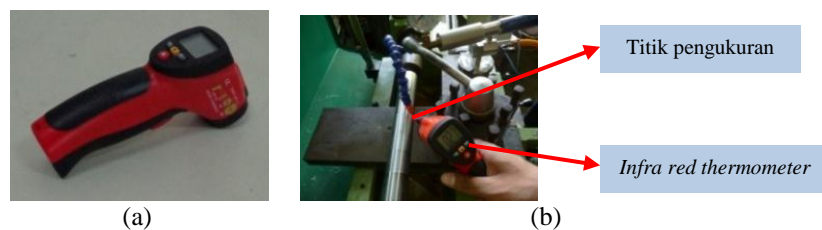
Gambar 6. (a) Infra red thermometer , dan (b) proses pengukuran temperatur pahat.
