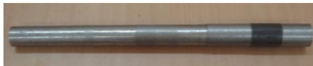
Gambar 1. Material benda kerja baja St 60.
