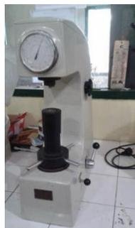
**Gambar 5.** *Rockwell Hardness Tester*
