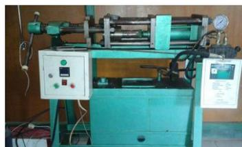
**Gambar 9.** High Pressure Die Casting (HPDC)
