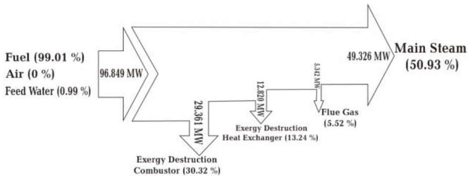
Gambar 17. Diagram Grassman Aliran Exergi Total di Boiler.
