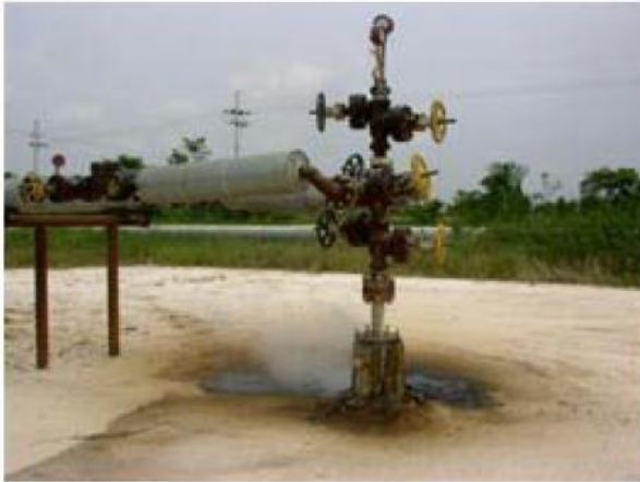
Gambar 3. Steam injector (injektor uap).
