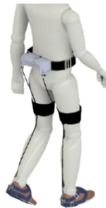
Gambar 1. Desain 3D ankle exoskeleton mekanisme cable-driven
