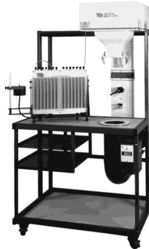
Gambar 2. Air flow bench dan Manometer
