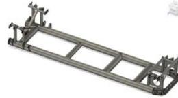
Gambar 3. *Ladder Frame Chassis*[10]
