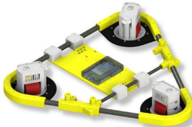
Gambar 7. Desain mekanisme chassis swerve wheel
