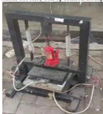
Gambar 5. Proses compression molding
