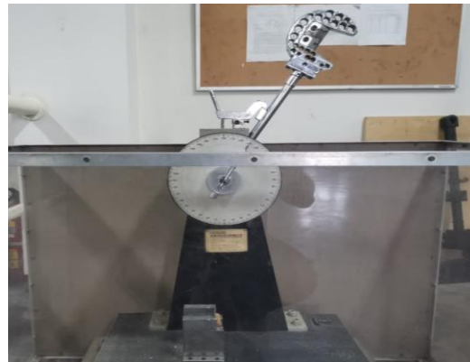
Gambar 7. Impact testing machine.
