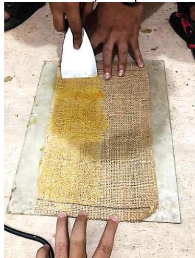
Gambar 3. Proses *hand lay-up*.
