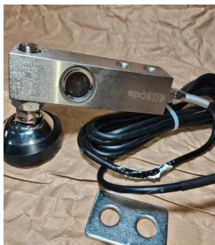
Gambar 9. (a) Load cell DSCells 250 Kg, (b) Spesification DSCell [10]
