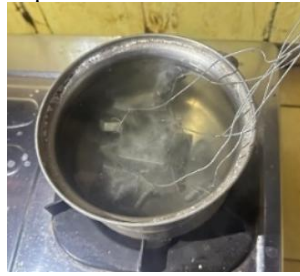
Gambar 8. spesimen sedang direndam didalam larutan zinc ammonium chloride .
