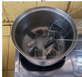
Gambar 6. spesimen sedang direndam didalam larutan water glass
