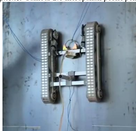
Gambar 1. Pengujian prototype magnetic crawler
