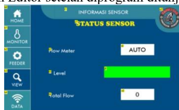
Gambar 6. Interface Nextion Editor setelah diprogram.
