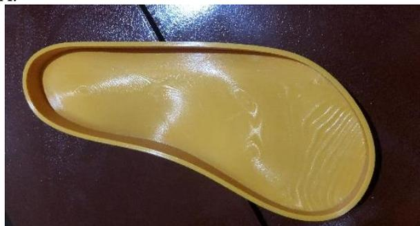
**Gambar 5.** Hasil Percetakan 3D Printing Moulding Insole
